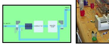
circuit sends effluent culture fluid back to the pump for recycling purposes, eliminating unnecessary waste.
